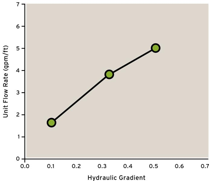
ClosureTurf was designed with the above characteristics in mind. The sand infill can handle **over six inches per hour of rainfall intensity without erosion** when applied on 3H:1V slopes.
