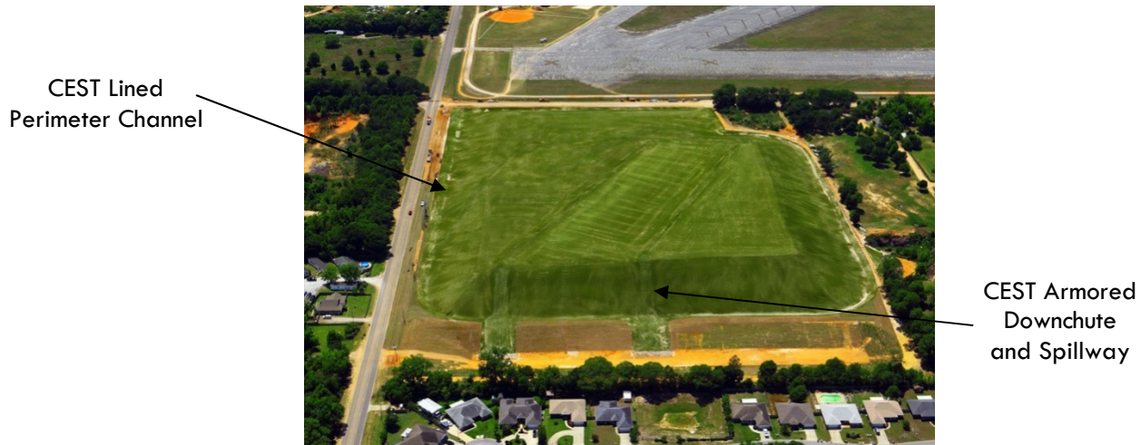
Figure 8: EST/CEST System in Service at the Saufley Field Road Landfill in Pensacola, FL
