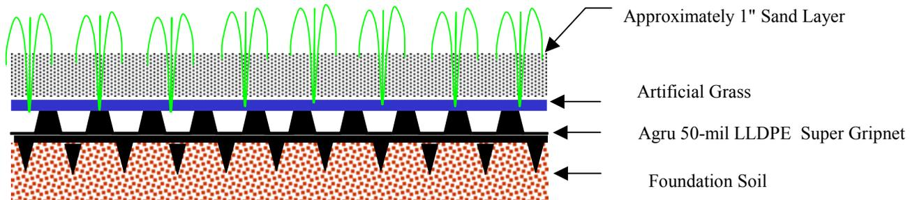
Figure 1. Cross-section of the Closure Turf system
