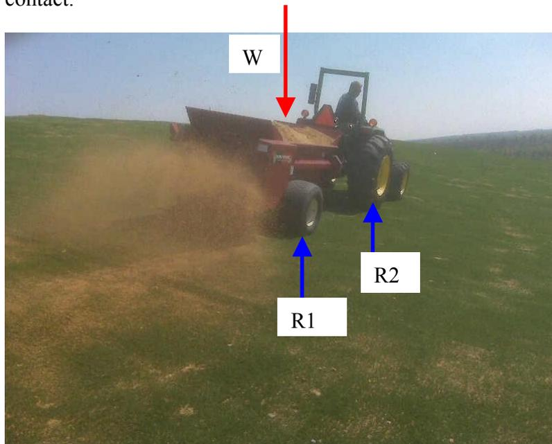
Figure 2. Rubber-tired construction equipment on the Closure Turf system.
