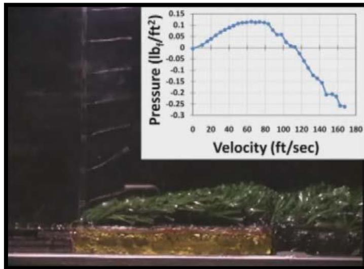
**Figure 2 – Aerodynamic Evaluation of HydroTurf at GTRI**
