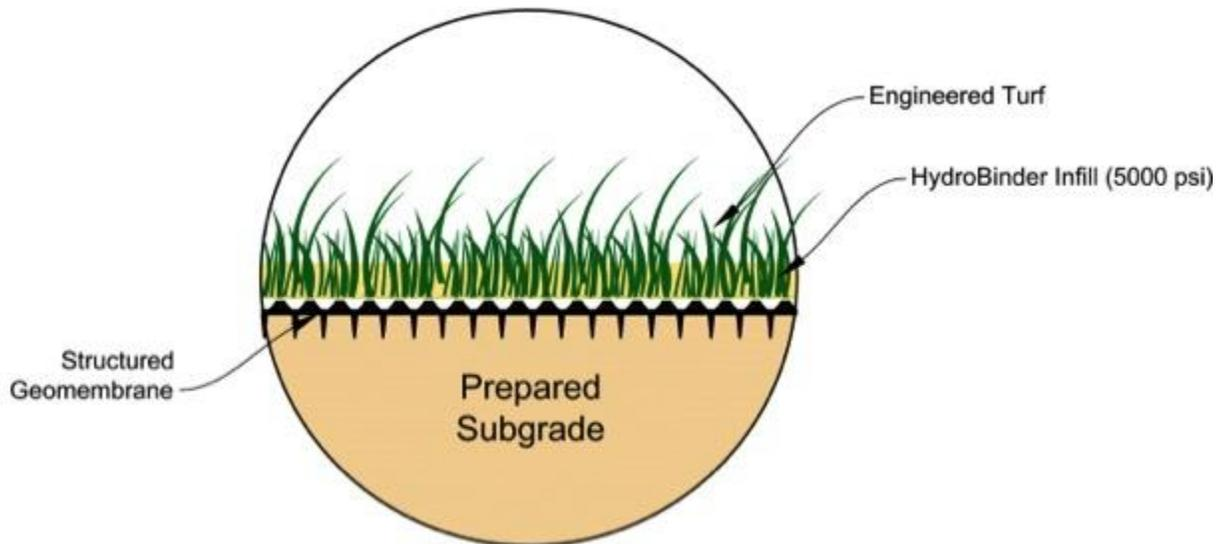
**Figure 1 – Section of HydroTurf® Revetment System**
