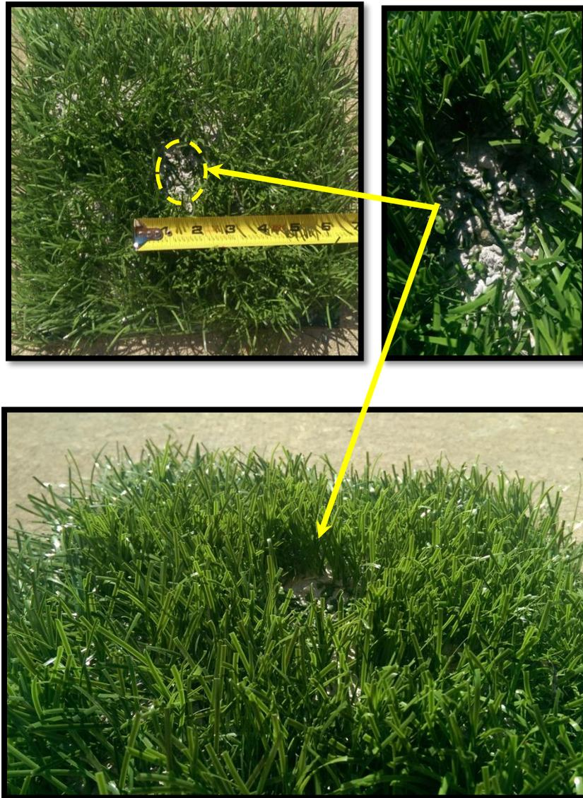
**Figure 6 – HydroTurf® Sample after Flammability Testing**
