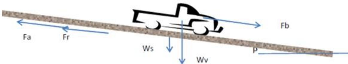
**Figure 8 – Schematic of Breaking Forces**
