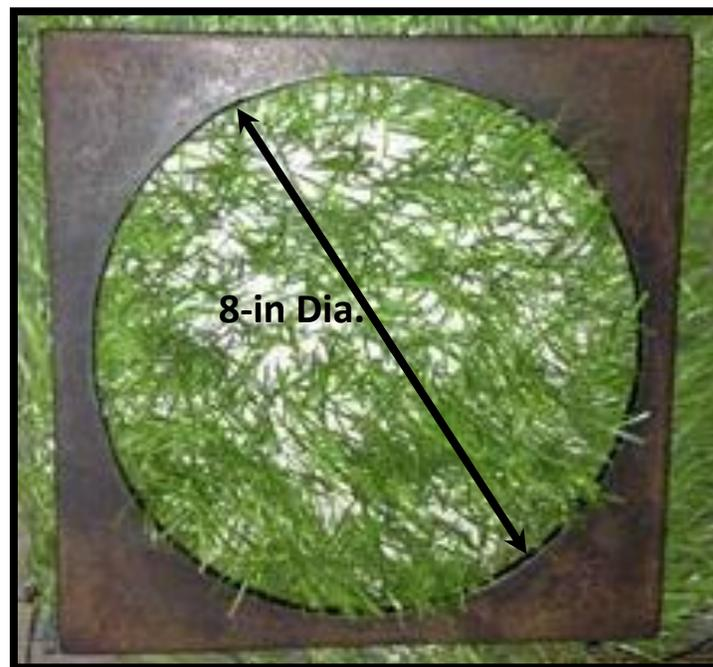
**Figure 5 – HydroTurf® Sample Prepared for Flammability Testing**
