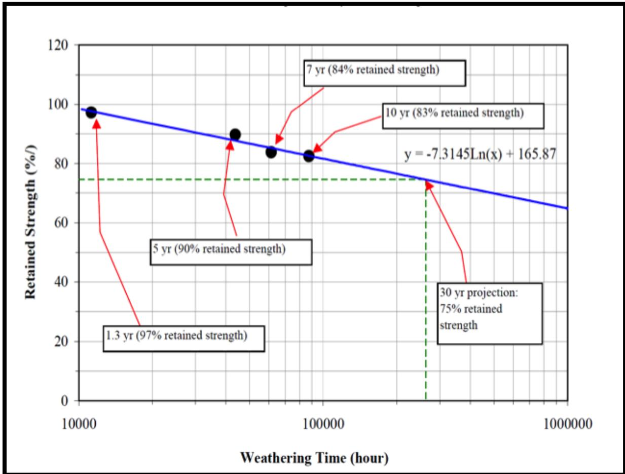
**Figure 4 –Retained Tensile Strength of Synthetic Turf Fibers vs. Weathering Exposure Duration**
