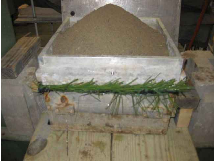
Figure 4. Concrete sand placed in the upper box on top of HydroTurf.
