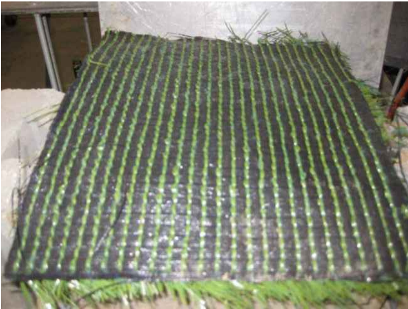
Figure 5. Bottom surface of HydroTurf after the completion of test.
