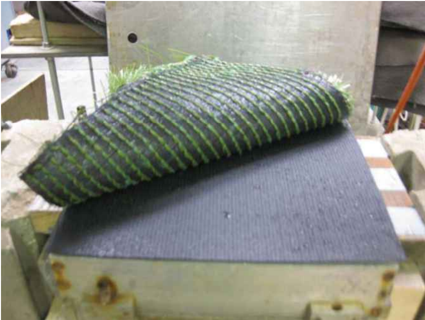
Figure 3. HydroTurf and geomembrane placed on top of compacted #57 stone.
