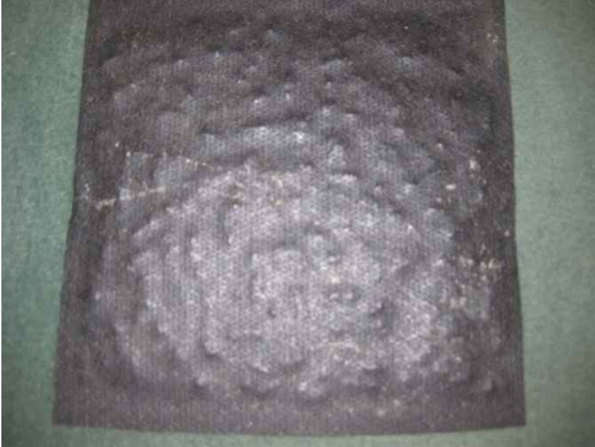
Figure 6. Deformed top surface of the geomembrane after the completion of test. No punctures or holes observed.
