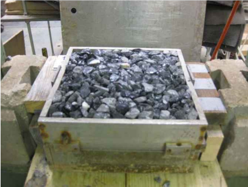
Figure 2. Compacted VDOT #57 stone in the lower box.
