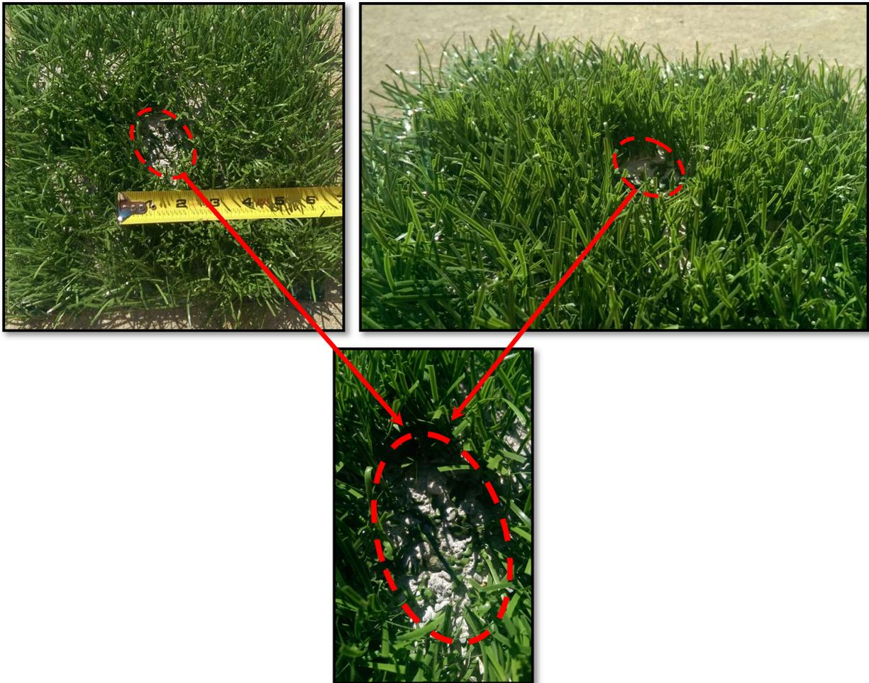
**Figure 2. HydroTurf® Sample after Flammability Testing**
