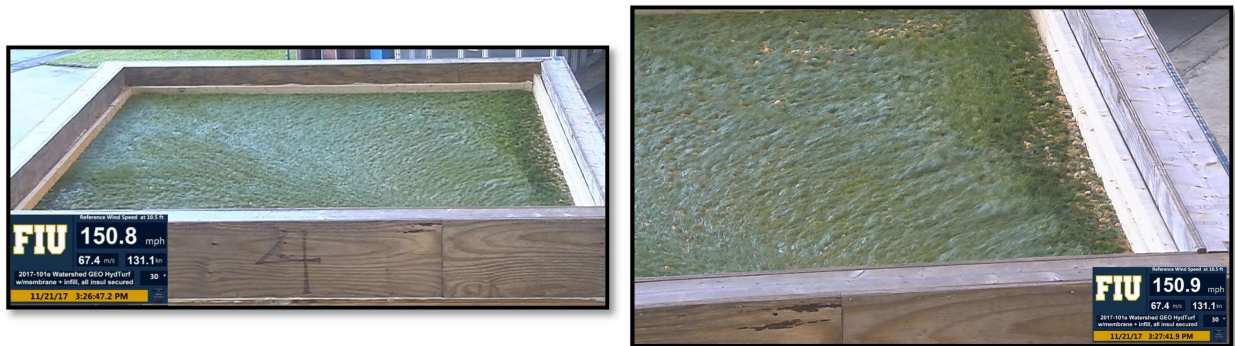
Figure 3. HydroTurf® Wall of Wind Testing in Progress
