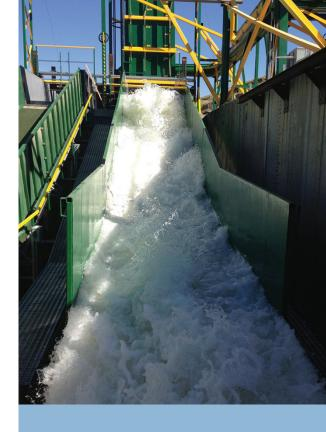
HydroTurf® has been comprehensively tested at Colorado **State University (CSU).** CSU's laboratory has the largest flumes for hydraulic testing in the world. HydroTurf did not reach failure at a maximum steady state overtop velocity of 40 feet/second and for 13 hours in the wave simulator overtop being subjected five-hundred-year hurricane event for the New Orleans region.
