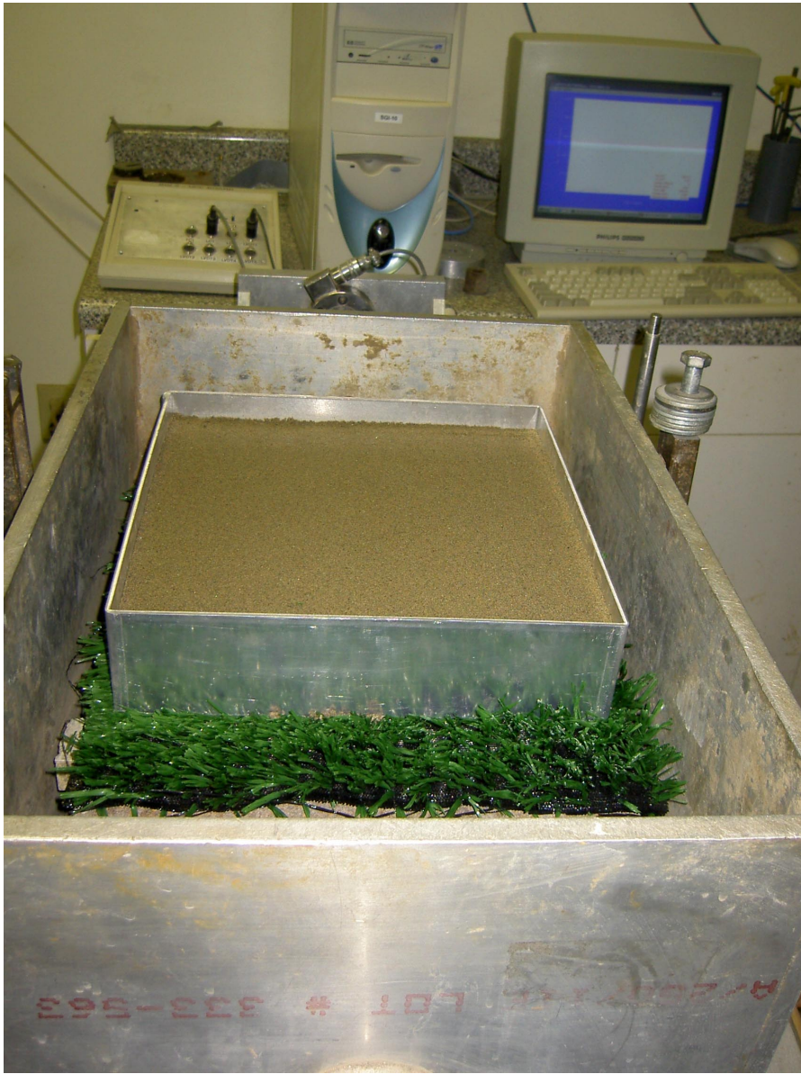
Figure 2. Sand/grass interface test at a normal stress of 20 psf.
