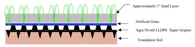
Figure 1. Cross-section of the Closure Turf system
