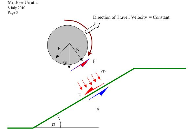
Figure 3. Tire-soil contact loading conditions on a slope. (NOTE: not to scale).
