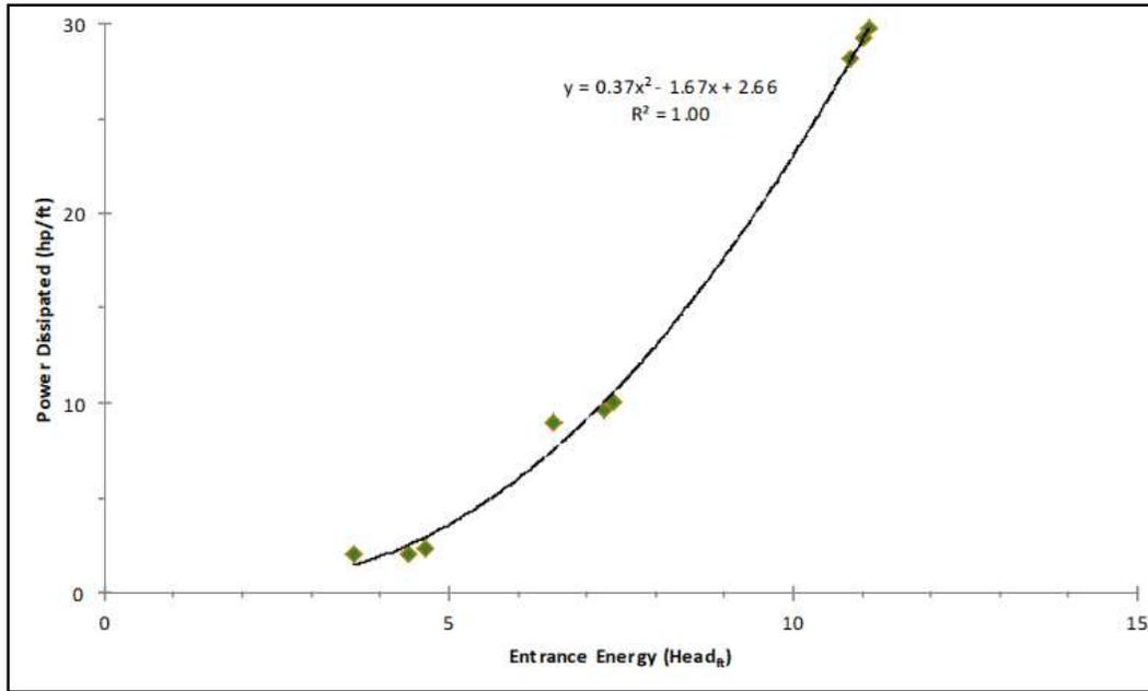
**Figure 12. HydroTurf® Hydraulic Jump Power Dissipation Results**
