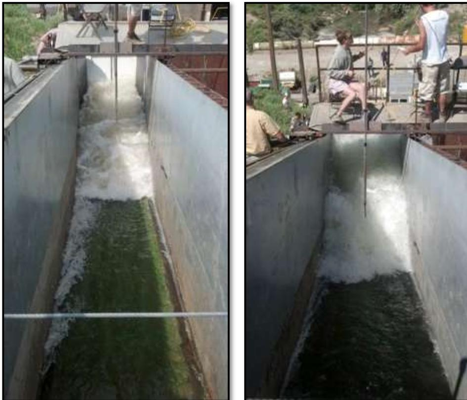
Figure 10. HydroTurf® Hydraulic Jump Testing at CSU
