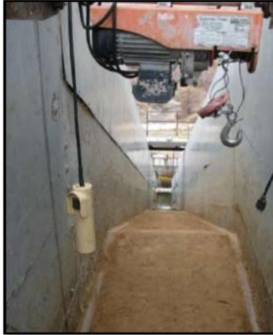
**Figure 2. Compacted Sandy-Loam Subgrade**
