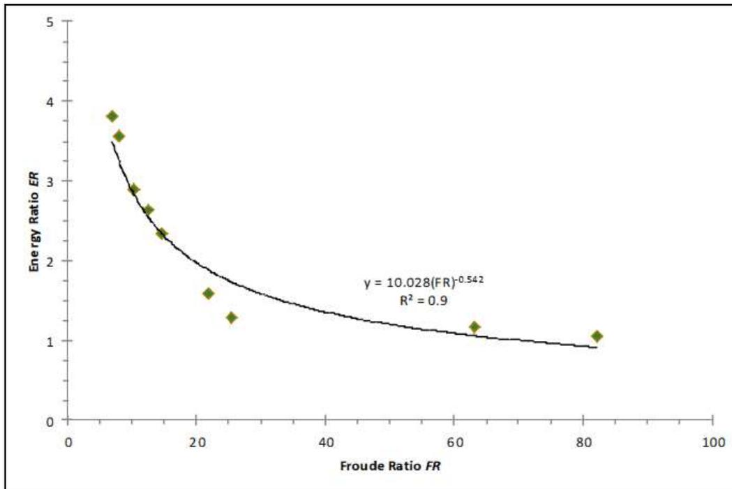
Figure 11. Energy Ratio as a Function of Froude Ratio for HydroTurf<sup>®</sup>
