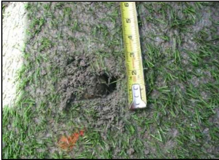
**Figure 17. Intentionally Damaged HydroTurf®, Pre-test**
