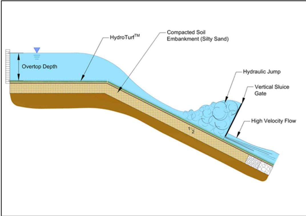
Figure 9. HydroTurf® Hydraulic Jump Testing Schematic
