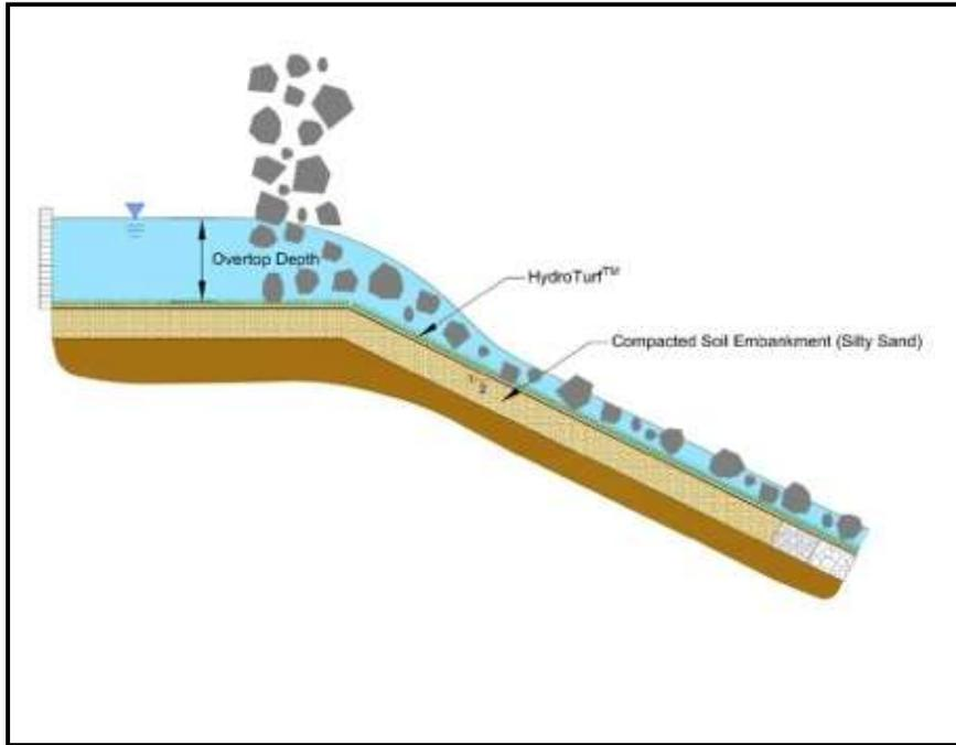
**Figure 15. Heavy Debris Load Testing Schematic**
