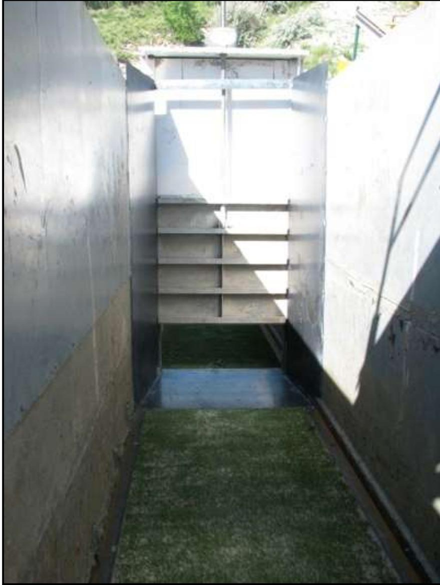
**Figure 8. Hydraulic Jump Testing Sluice Gate Installation**
