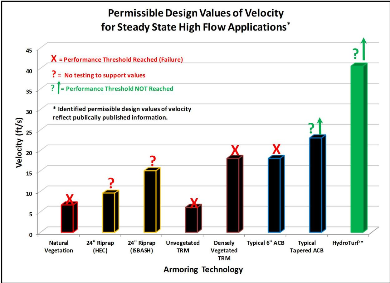
**Figure 7. Accepted Velocity Design Values for Steady State, High Flow Applications**
