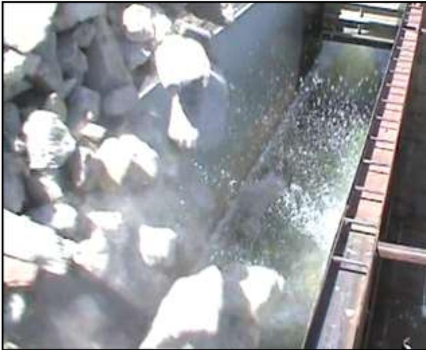
**Figure 16. Heavy Debris Load Evaluation (Concrete Rubble)**
