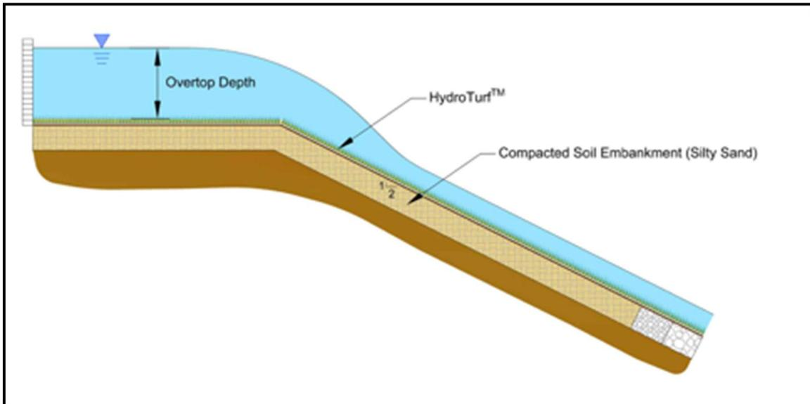
**Figure 5. HydroTurf® Overtopping Testing Schematic**
