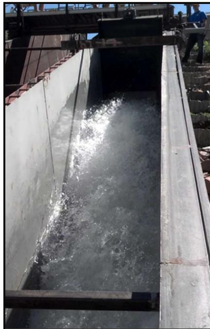
**Figure 13. Pressurized “Jet” Impinging on HydroTurf®**
