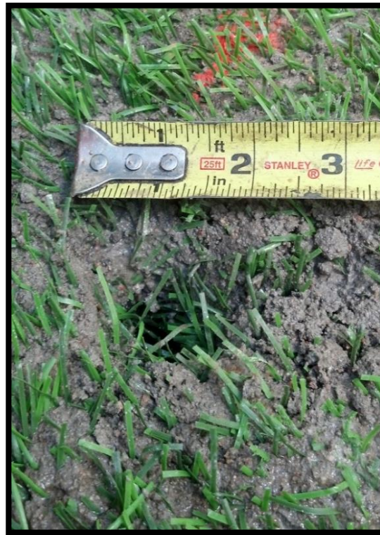
Figure 13: Intentional Hole in the CEST Prior to Testing
