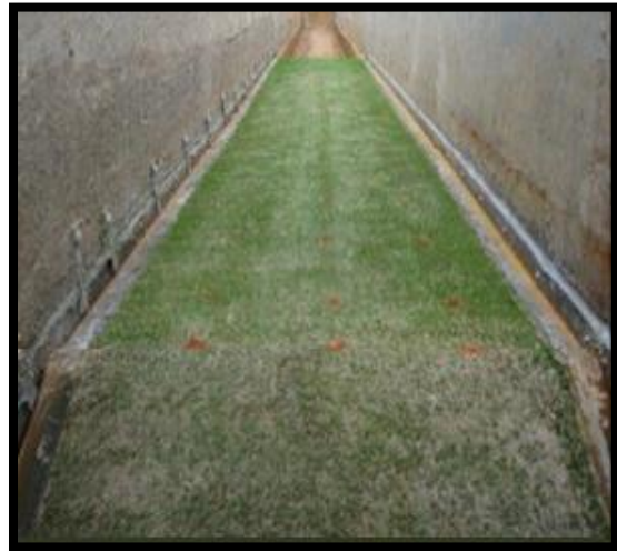
Figure 4 – Completed Installation of the CEST Prior to Testing
