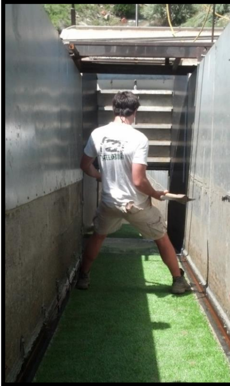
Figure 12: Pickaxe Being Used to Create an Intentional Hole
