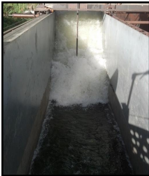
Figure 8: Hydraulic Jump Testing of the CEST
