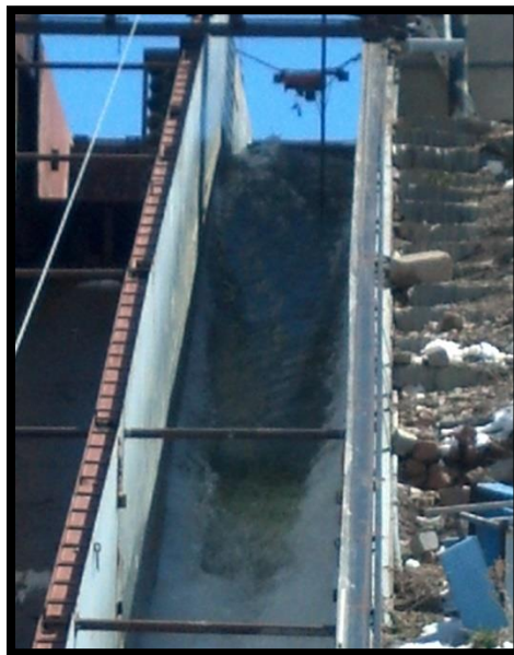
Figure 7: CEST Testing of 5 Foot Overtopping Depth in Process
