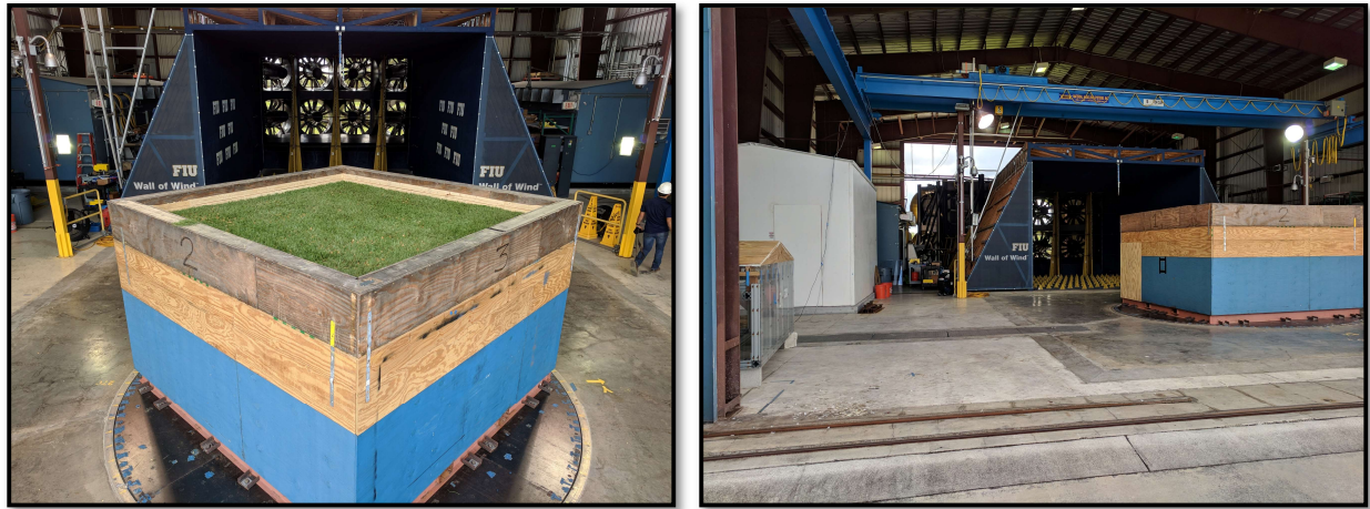
Figure 1: ClosureTurf® Wall of Wind Test Installation
