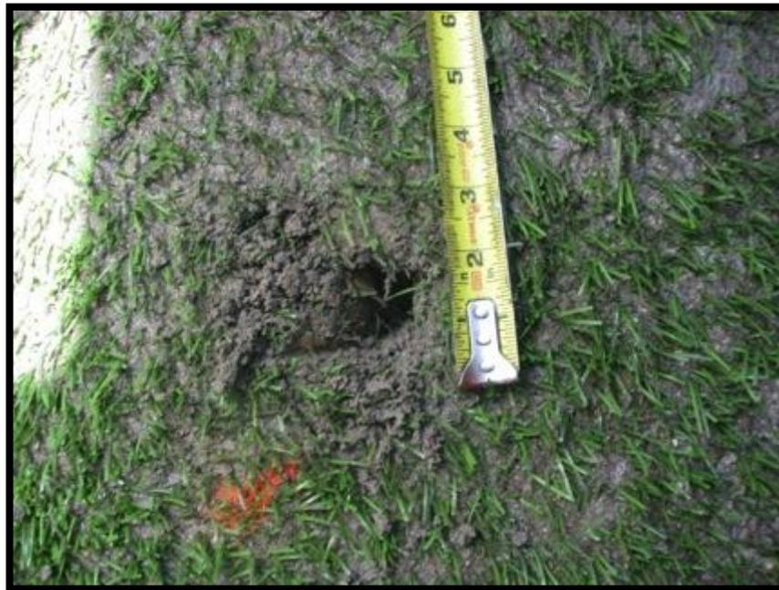
**Figure 17 - Intentional Damage: Hole from Pick Ax
