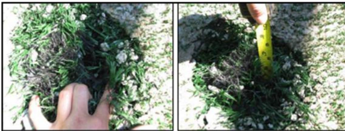
**Figure 25 – Intentional Damage: Large Hole through HydroTurf®**
