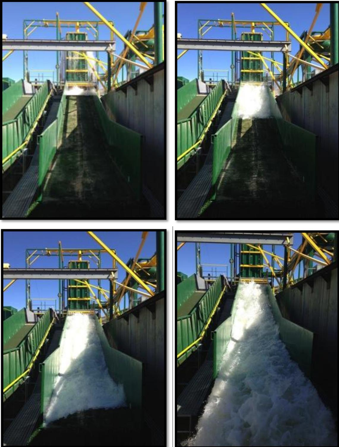
**Figure 26 – Wave Overtopping Testing of HydroTurf® at CSU**
