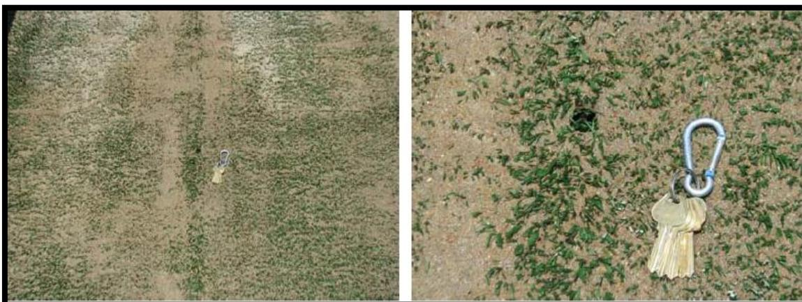
**Figure 24 – Intentional Damage: Simulated Bullet Hole through HydroTurf®**
