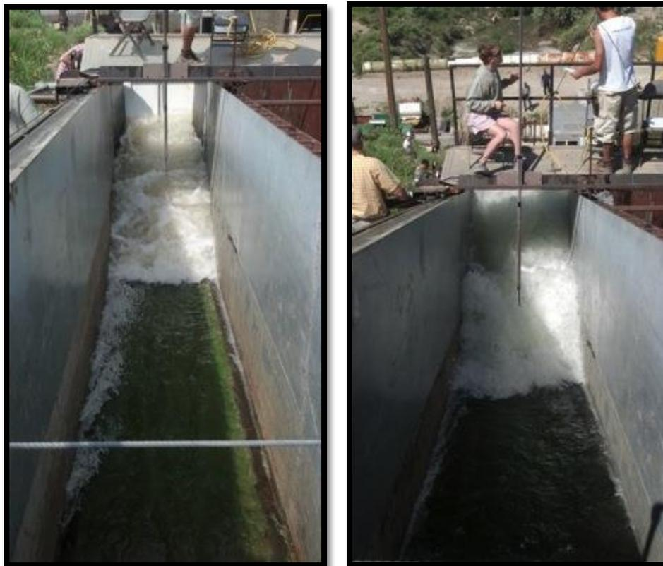
**Figure 10 – Hydraulic Jump Testing of HydroTurf® at CSU**
