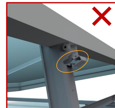
LOCK CLAW NOT INSTALLED
