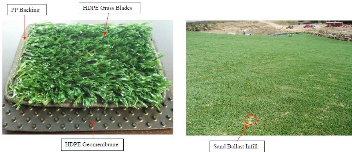
Figure 1. Typical engineered turf components.
