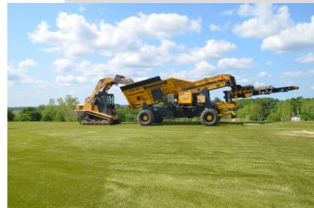
Rubber tired vehicles can be driven on ClosureTurf® without risk of damage.
