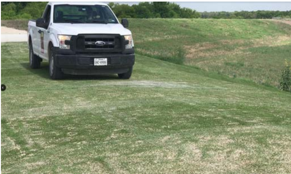
As part of the post-construction sign-off, the contractor was required to perform a traffic loading test over HydroTurf. A typical maintenance vehicle was driven across the HydroTurf twenty (20) times during dry and wet conditions. No damage to the system was noted due to the vehicle loading.
